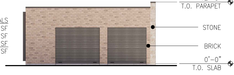
BLDG C SOUTH ELEVATION SCALE: 3/32" = 1'-0"
