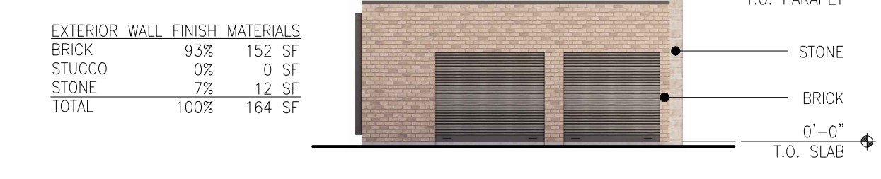
BLDG C EAST ELEVATION SCALE: 3/32" = 1'-0"
